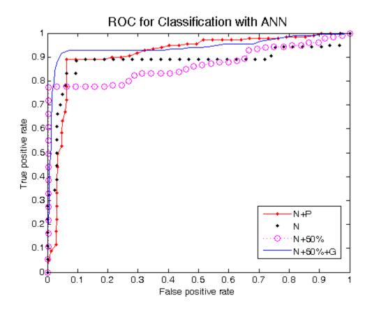
Figure 18. ROC curves for N, N+P, N+50%, and N+50%+G CAD tools. The N+50%+G ROC curve (blue) shows better performance than the N (black), N+P (red), or N+50% (purple) ROC curves.
