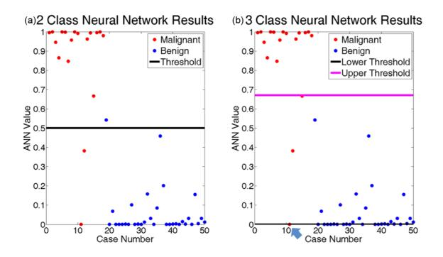
Figure 20. The neural network values for the N+50%+G experiment. The values of the network are plotted against the case number; correct diagnosis is indicated by the color of the point. The threshold(s) is(are) shown in black and magenta. (a) shows a single threshold/two class division. (b) shows the two threshold/three class division. Due to case 11 (see blue arrow in (b)), the lower threshold is set at 0.
