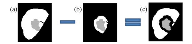
Figure 14. Construction of peel mask. (a) the larger parenchyma mask (in white), in this illustration the 40% mask, is selected for the outer bounds of the parenchyma mask. The parenchyma mask to be removed (b, also in white), the 10% mask, is subtracted from (a), leaving the outer peel of parenchyma (c). The nodule volume is shown in grey in (a)-(c).
