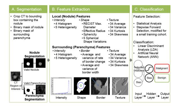
Figure 4. Flowchart of the computer-aided diagnosis tool. The region of interest containing the nodule and surrounding parenchyma is labeled as nodule or parenchyma (A. Segmentation). In B. Feature Extraction, over 300 features are extracted from these two areas. Finally, the feature set is reduced and the selected features are used to train the neural network classifier (C. Classification), labeling a nodule as likely malignant or likely benign.
