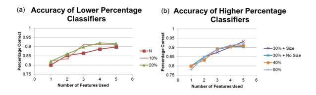
Figure 16. Classifier performances as the number of features included is increased. In (a), the accuracies of the lower percentage classifiers tend to level off after 3 features are used for classification. However, for the higher percentage classifiers (b), the only percentage that continues to increase with more features is the 30%+size mask. The 40% and 50% masks' performances level off after 4 features, respectively.
